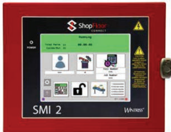
RIGHT: The network-ready and factory configured ShopFloorConnect Machine Interface (SMI 2) connects virtually any machine to the ShopFloorConnect Machine Monitoring Software.
