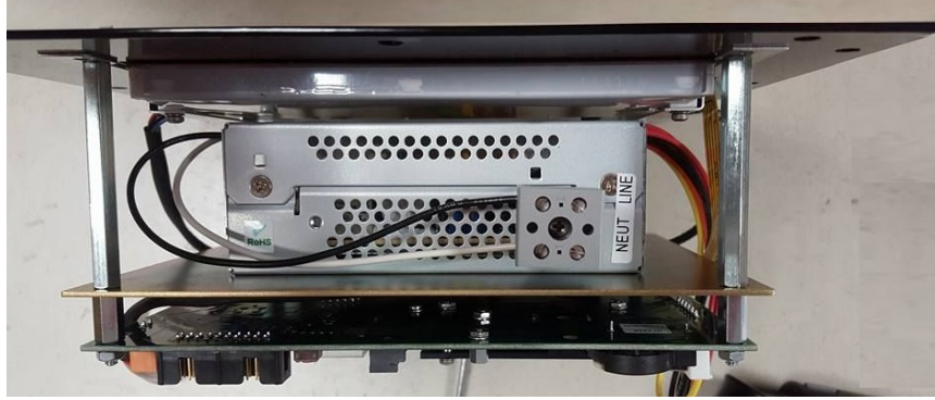
Figure 2-6. AC Wiring on SMI 2 Panel Mount
