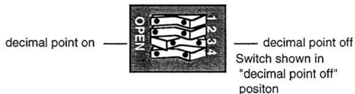
Figure 3-3. Setting decimal point switch on calibration unit
