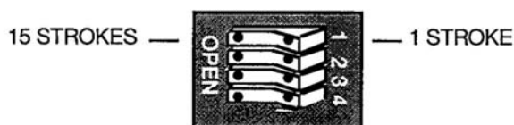
Figure 4-1. Stroke select switch (#1) with 15 strokes selected
