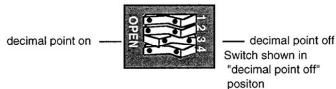
Figure 3-6. Switch block S101 showing decimal point switch
