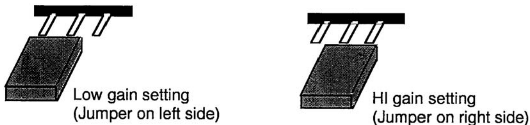
Figure 3-8. Jumper position for low gain and high gain
