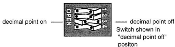
Figure 3-6. Switch block S101 showing decimal point switch
