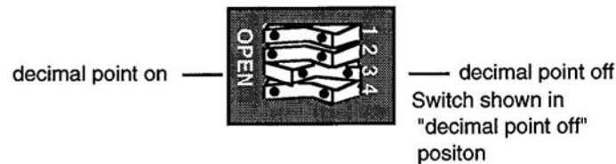
Figure 3-6. Switch block showing decimal point switch
