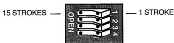
Figure 4-1. Stroke select switch (#1) with 15 strokes selected
