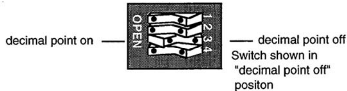
Figure 3-3. Setting decimal point switch on calibration unit
