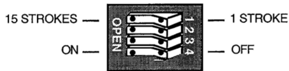
Figure B-1. Stroke select switch (S1) with on-off positions for switch 4 shown The following chart shows how to set dip switches 1 and 4 for 1, 15, 30 or 60 stroke settings:
