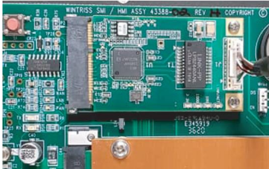
Figure 2. Mini PCIe NIC Module Inserted into P2 Connector
