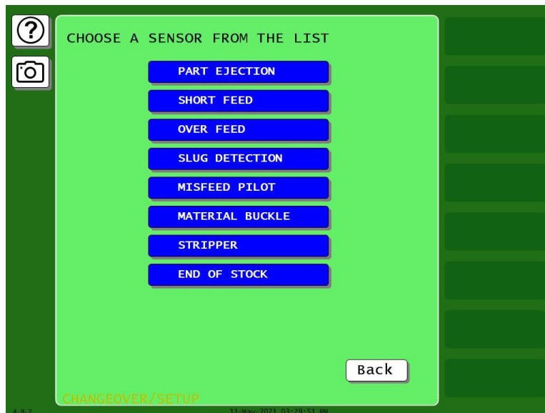
Figure 6-23. This Tool's Previously Programmed Sensors from Which You Can Copy the Timing and Stop Type
