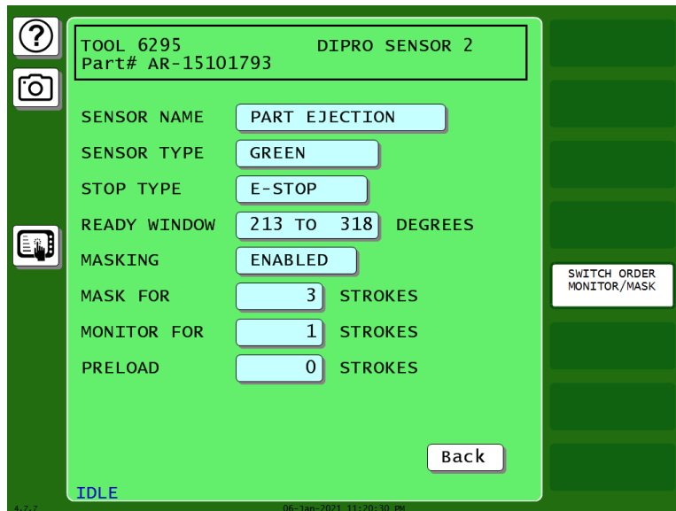
Figure 6-21. Standard Green Sensor Type with Masking Enabled.
