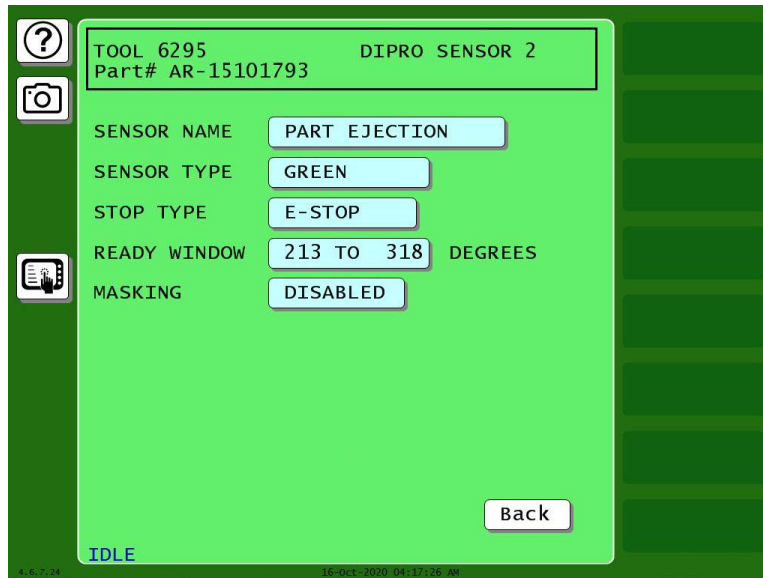
Figure 6-20. Sensor Program Screen showing the Masking feature disabled (default setting)
