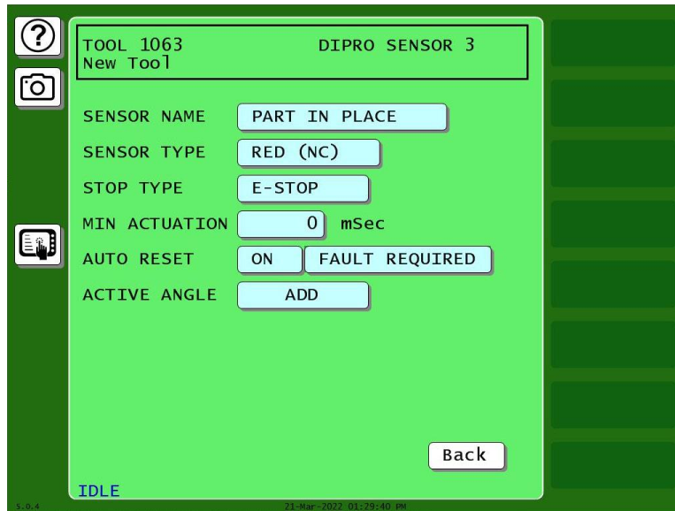
Figure 6-11. FAULT REQUIRED Enabled
