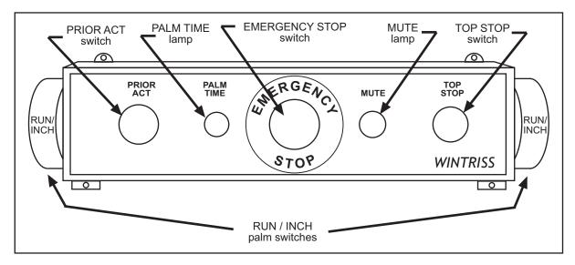
Figure 1-2. Operator Station Components (Side-mounted Run/Inch Palm Buttons)
