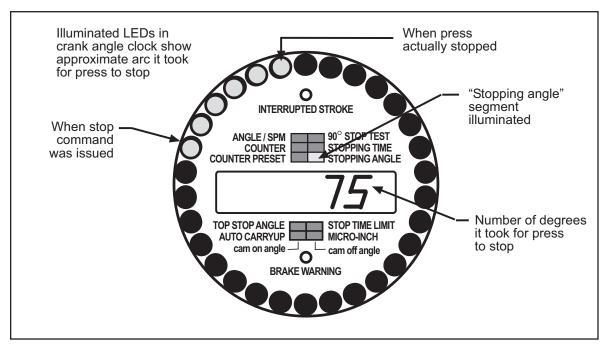
Figure 4-1. WPC 2000 Display with "Stopping Angle" Value Shown
