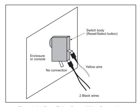
Figure 2-31. Reset/Select Button Wiring Connections
