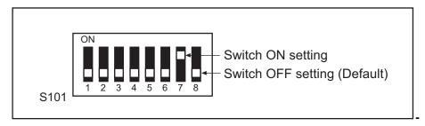
Figure 3-11. S101 Option Switch OFF and ON Settings
