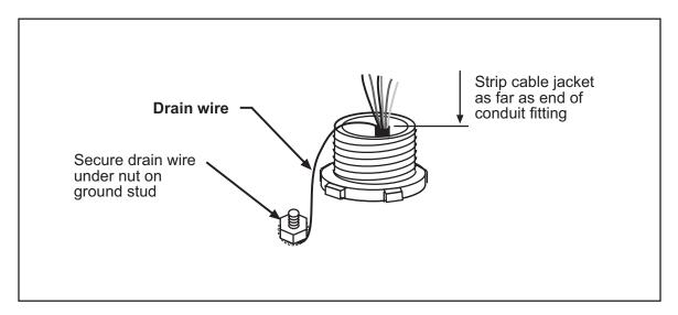
Figure 2-3. Cable Shield Termination
