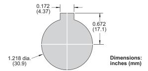
Figure 2-29. Selector Switch: Cutout Dimensions
