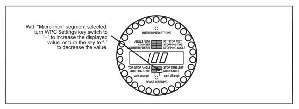
Figure 3-10. WPC 2000 Display Showing Micro-inch Time Setting
