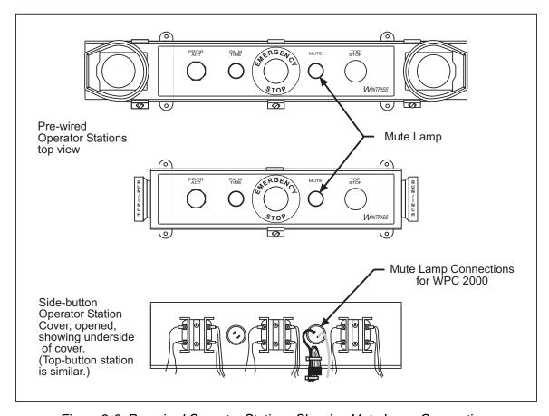
Figure 2-6. Pre-wired Operator Stations Showing Mute Lamp Connections
