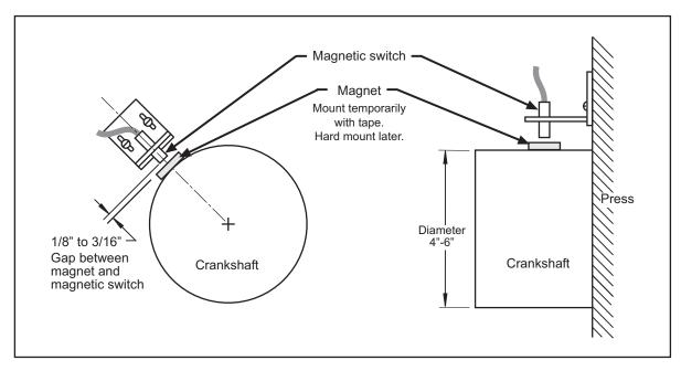
Figure 2-15. Overrun Sensor Magnetic Switch: Installation Example
