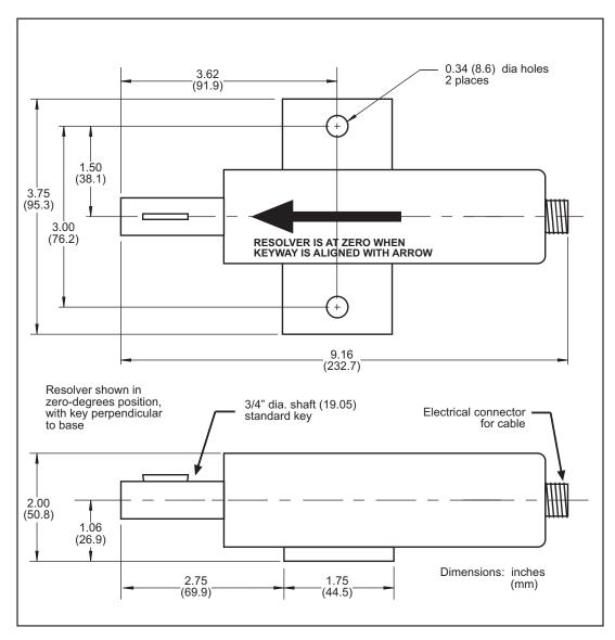
Figure 2-11. Resolver: Mounting Dimensions
