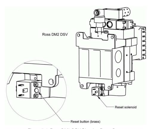
Figure 5-4. Ross DM2 DSV Showing Reset Button
