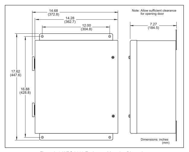
Figure 2-4. WPC 2000 Enclosure: Mounting Dimensions
