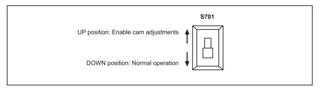
Figure 2-22. "Set Cams" Switch (S701) Positions
