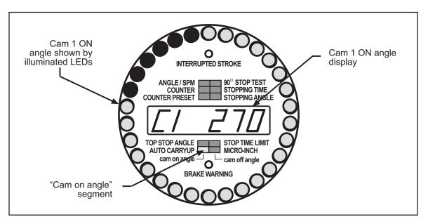
Figure 3-12. Cam Channel Settings Display: Cam 1 ON Angle (270°) Shown
