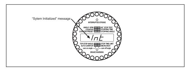
Figure 3-2. WPC 2000 Display Showing "System Initialized" ("Int") Message
