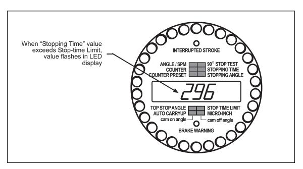
Figure 5-3. WPC 2000 Display Showing Stopping Time Fault
