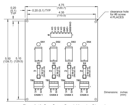
Figure 2-18. Cam Output Board: Mounting Dimensions
