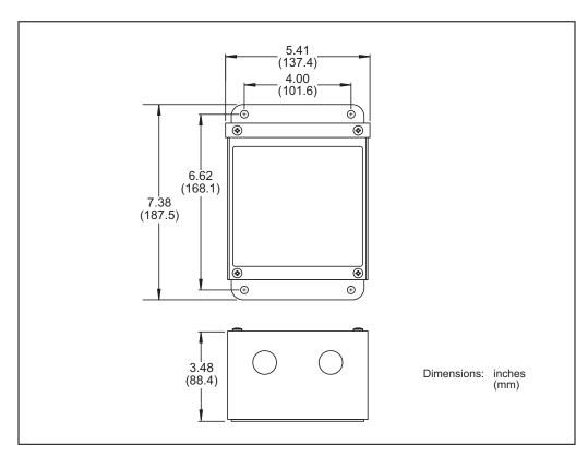
Figure 2-17. Cam Output Enclosure: Mounting Dimensions
