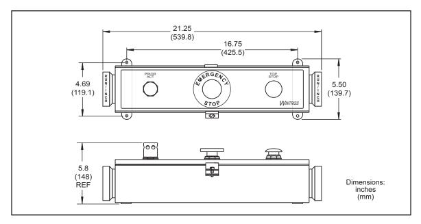
Figure 2-10. Unwired Operator Station: Mounting Dimensions
