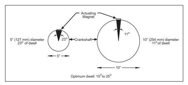
Figure 2-14. Overrun Sensor Magnet Placement: Dwell as a Function of Shaft Diameter
