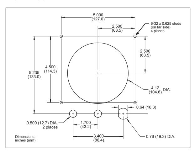
Figure 2-30. WPC 2000 Display Board Kit: Mounting and Cutout Dimensions
