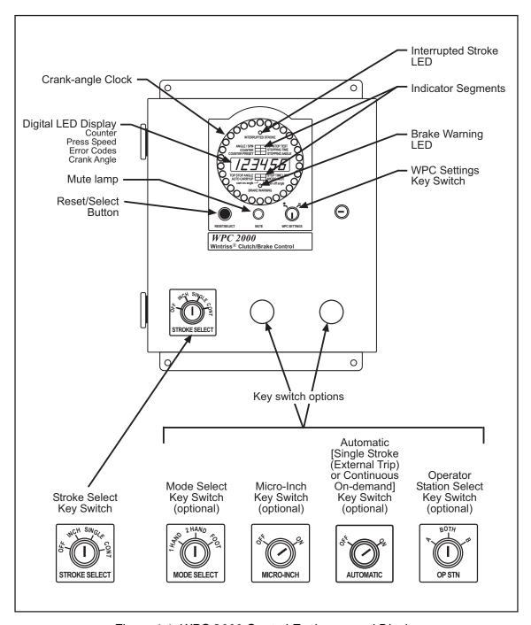
Figure 1-1. WPC 2000 Control Enclosure and Display
