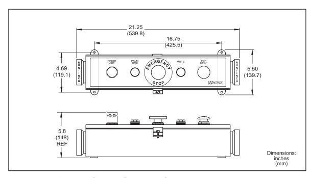
Figure 2-8. Pre-wired Operator Station with Side Run Buttons: Mounting Dimensions
