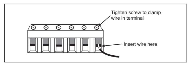
Figure 2-2. Correct Way to Attach Wires to Terminal Block Connectors
