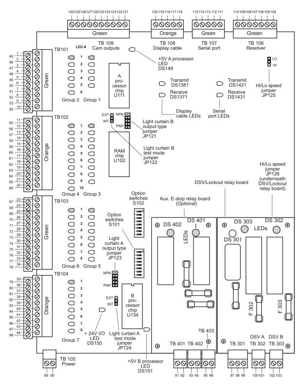
Figure 2-13. WPC 2000 Main Processor Board (Left Configuration):
