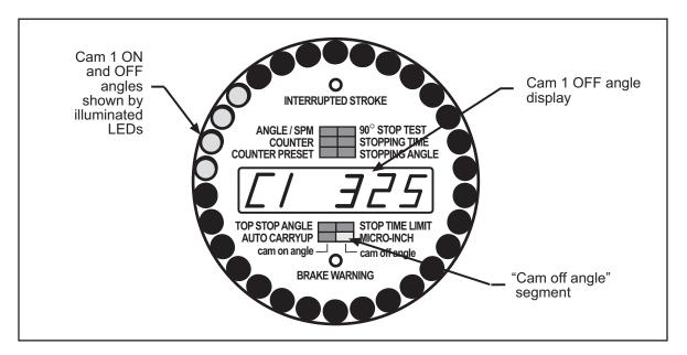
Figure 3-13. Cam Channel Settings Display: Cam 1 OFF Setting (325°) Shown
