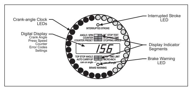
Figure 3-1. WPC 2000 Display Showing Indicator Segments
