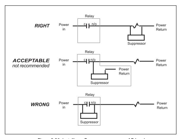
Figure 2-20. Installing a Suppressor across an AC Load
