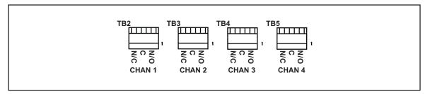
Figure 2-19. Connectors TB2 through TB5 on Cam Output Board
