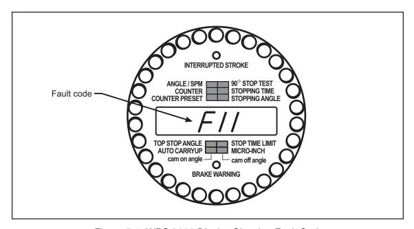
Figure 5-1. WPC 2000 Display Showing Fault Code
