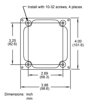
Figure 2-24. One-hand Control Switch Base: Mounting Dimensions
