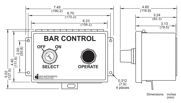
Figure 2-26. Bar Control Enclosure: Mounting Dimensions
