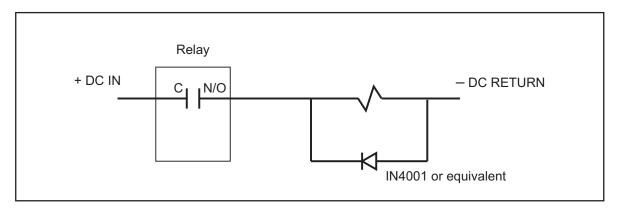
Figure 2-21. Installing a Diode across a DC Load
