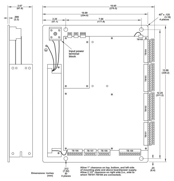
Figure 2-27. WPC 2000 Mounting Plate: Mounting Dimensions
