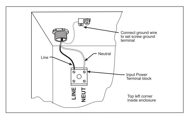
Figure 2-5. AC Input Wiring Connections
