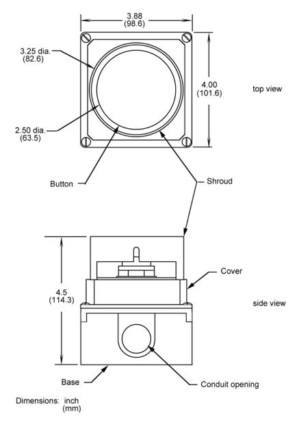
Figure 2-23. One-hand Control Switch: Mounting Dimensions
