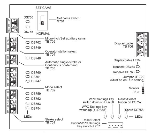
Figure 2-16. WPC 2000 Display Board: Location of Important Components
