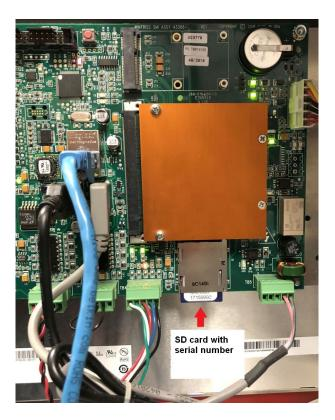
Figure 2-22. SmartPAC PRO SD Card with Serial Number on HMI Board
